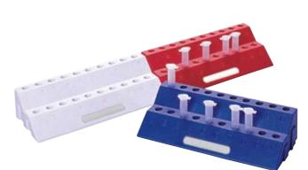
Polypropylene racks for storing 20 tubes. Racks lock together on each side.
