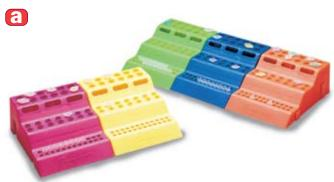
Three way polypropylene racks connect to one another on either end. Convenient finger slots are moulded onto the rack and each of the three tiers accommodates a different size tube. Lowest level has 24 wells to hold individual 0.2mL tubes or strips of 8 or 12 tubes. The middle tier has 14 wells to hold 0.5mL tubes. The top tier has 12 wells to hold 1.5mL tubes. Autoclavable. Rack measures 164mm x 123mm x 62mm and is supplied in assorted colours (blue, green, purple, yellow, and orange).
