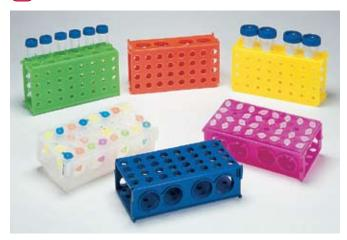
Four way heavy duty racks feature a unique system of tabs and slots which when linked together create a large rack.
