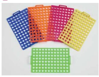
Save time when working with individual 0.2mL tubes or strips of 8 or 12 tubes.
