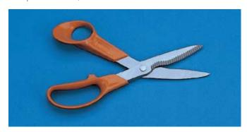
High quality scissors suitable for cutting polyester and aluminium backed TLC plates, whilst the glass knife is suitable for cutting glass backed TLC plates.
