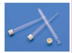
Test tubes, borosilicate glass, round bottom, screw thread without caps, disposable
