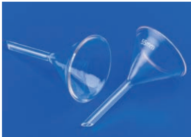
Funnels, borosilicate glass, conical, plain
